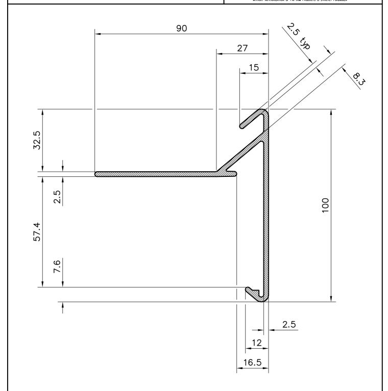
SUPPLIED IN 2.5 METRE LENGTHS WITH LOOSE JOINTING SLEEVE 90° INTERNAL AND EXTERNAL CORNER PIECES AVAILABLE STANDARD COLOURS BLACK, WHITE AND GREY OTHER COLOURS CAN BE SUPPLIED, PRICES & LEAD TIMES ON APPLICATION
